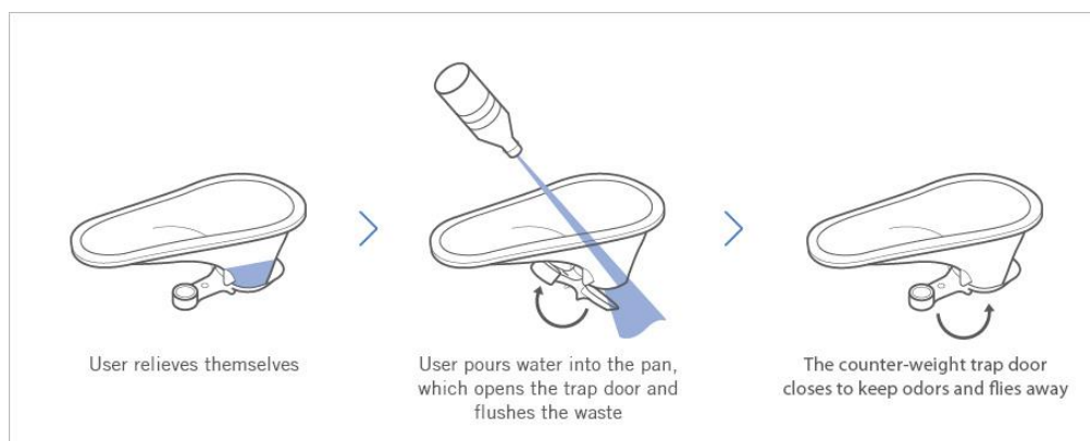
Diagram of a SaTo Pan toilet, Global Sanitation and Hygiene, Lixil (2019)
